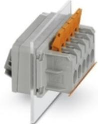
Panel feed-through terminal block, connection method: Push-lock connection, Push-in spring connection, number of positions: 4, load current: 41 A, cross section: 2.5 mm<sup>2</sup> - 10 mm<sup>2</sup>, connection direction of the conductor to plug-in direction: 0 °, width: 64.4 mm, color: gray
